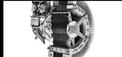
In 1912, Siemens Brothers' success was helped by the Uniselect, an electro-mechanical stepping switch that automatically connected calls. It sped up telephone exchanges – but reduced the need for switchboard operators.
